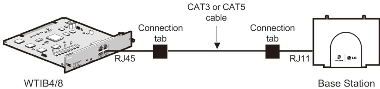
Figure 3.5-2 Wiring with connection tab between WTIB4/8 and Base Station
