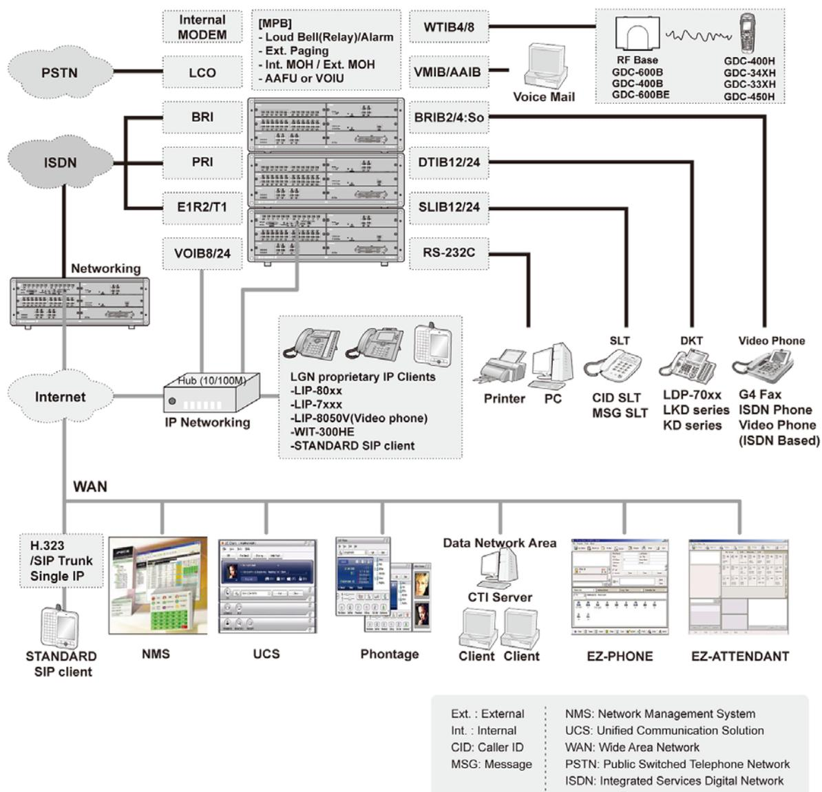
Figure 1.1-1 System Connection Diagram
