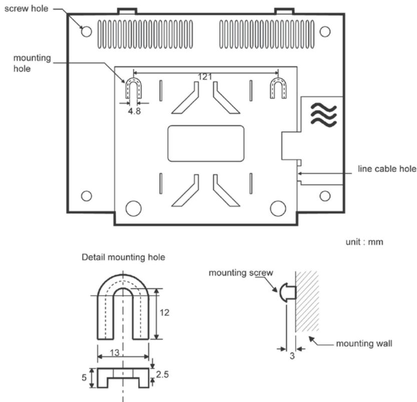
Figure 3.4.2.1-1 GDC-400/600B (Rear View)
