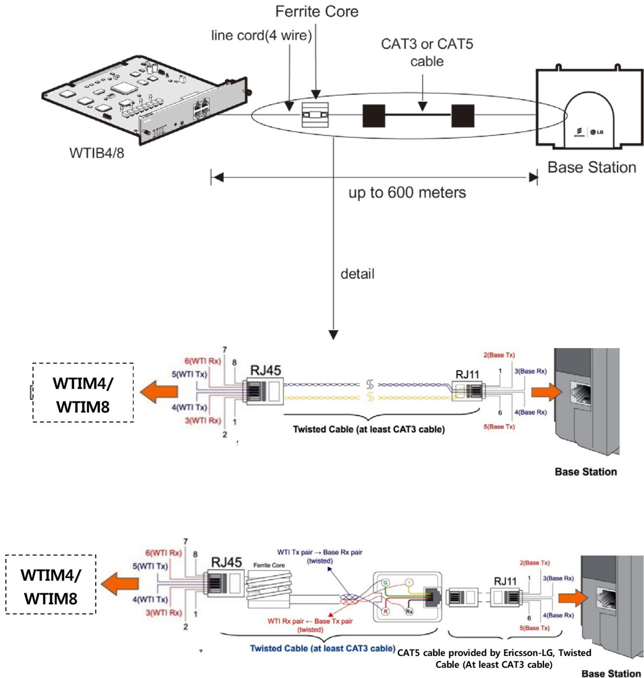
Figure 3.5-1 Cable connection with Ferrite Core between WTIB4/8 and Base Station
